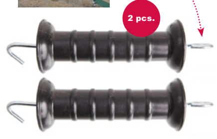
Heavy-duty gate handle with compression string. In the heavy-duty gate handle, instead of elongation, the spring is compressed in a closed space inside the handle. Lasts clearly longer than a standard gate handle without breaking.
