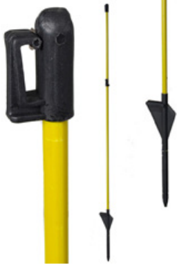
Traditional yellow fibreglass post with two insulators included. The position of the lower one can be changed. Fibreglass post insulators can be used as spare insulators. The post surface structure efficiently prevents sticking. Fibreglass posts can be used with fence wires and fence tapes of maximum width 20mm. Three lengths:
