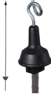
The spring steel post is a fence post made of durable spring steel with a pigtail insulator at its end. Fibreglass post insulators can be used as spare insulators. Spring steel posts can be used with fence wires, fence ropes, and fence tapes of maximum width 20mm. Two lengths:: • Length 142cm, above-ground length 124cm • Length 108cm, above-ground length 90cm.
