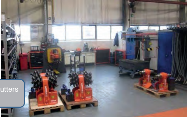
Final assembly station of the grabs - customized assembly -
