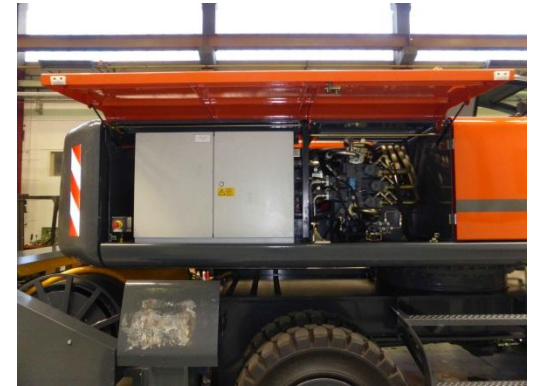
Control cabinet and distributor block
